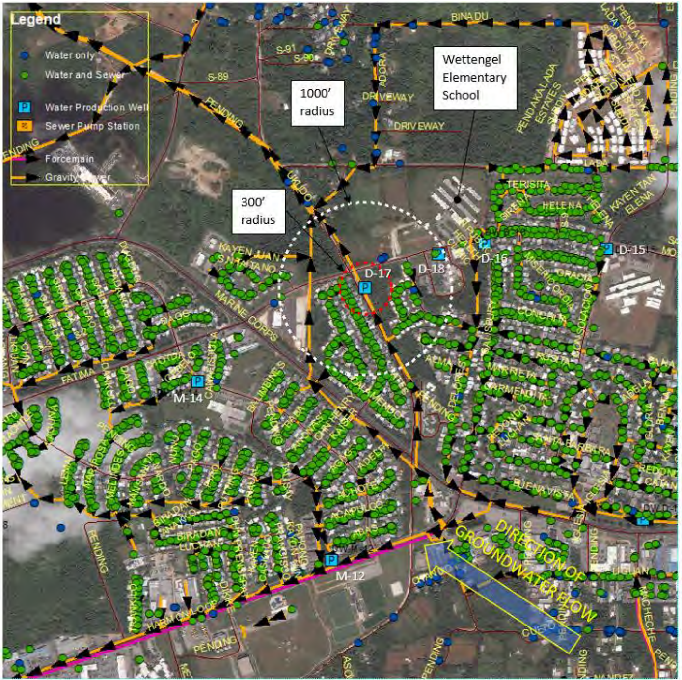
Figure B4. Well D-17’s high concentration levels may be attributed to faulty surrounding sewer infrastructure. Sewer mains will be investigated with the latest CCTV data and input from Operations and Maintenance to determine areas needing repair, rehabilitation, or replacement. Although current test samplings of wells D-18 and D-16 to the east indicate relatively lower nitrate-nitrogen concentration levels, their proximity to an elementary school and well D-17, taking into account future drawdown and zone of influence of the water table in well pumping, only adds to the area’s importance.
