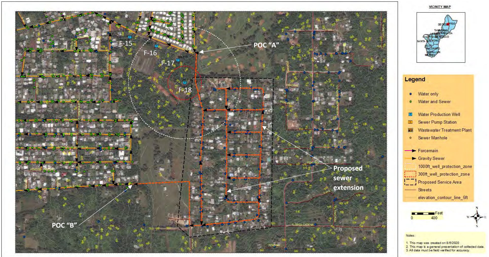
Figure 25. Map of Proposed sewer extensions in the Piga subdivision near wells F-18, F-17, F-16, and F-15. The points of connection to the existing sewer system (POC) are identified.
